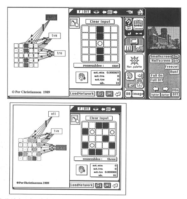
Fig. 16. A background agent in the form of a neural net is integrated into the HyperCard stack. Pattern can be recognized. For clarity the Hopfield network which was trained outside HyperCard recognizes a "one" and "three" pattern. The missing input squares are marked in the figure (circles). The net is normally not displayed on the screen. (In the upper right corner is a reduced videodisk overlay image.)
