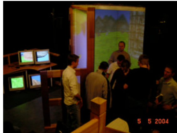
FIG. 3: The 6 sided CAVE at the VR Media Lab at Aalborg University provides total visual and audio surrounding for small groups to experience and manipulate virtual worlds.
