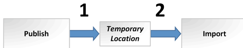
Figure 246 – Vico’s Two Step Process: publish data from Constructor into a temporary location in the database and then import it when you need it.
