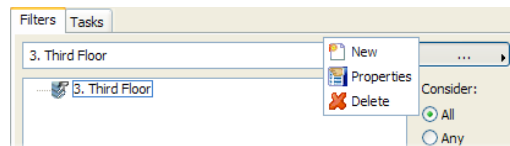
Figure 384 – Using the Filter Set Function Button to create, edit or delete a filter set.
