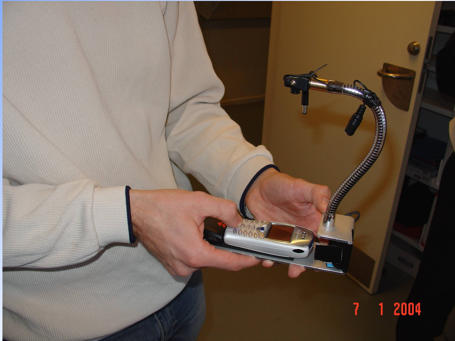
Ericsson T68i Mobile phone mounted on video stand for capture of mobile phone keyboard and screen. The video camera is wirelessly connected to video recording device.
