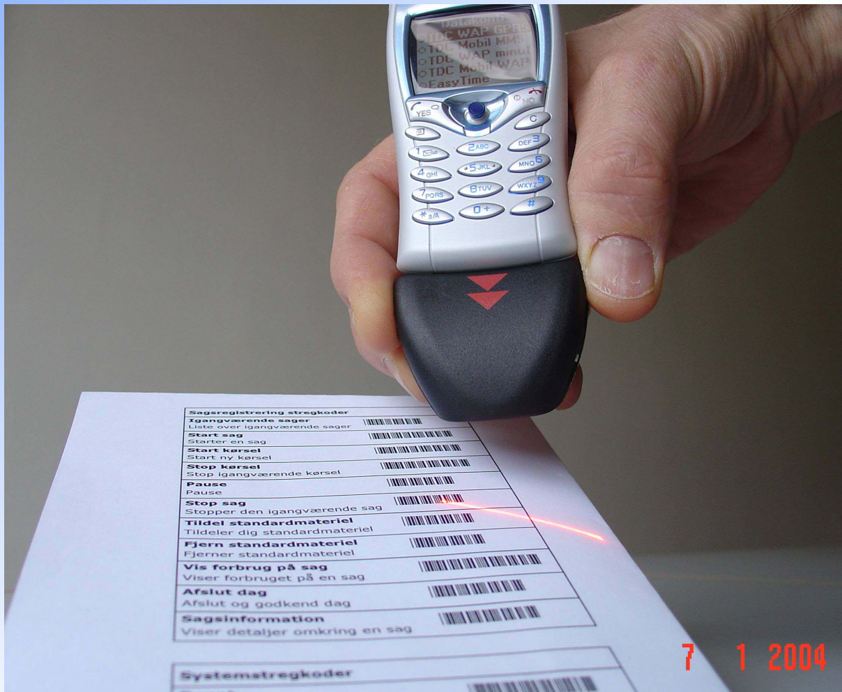
Ericsson T68i Mobile phone equipped with barcode reader scanning a laminated barcode sheet.
