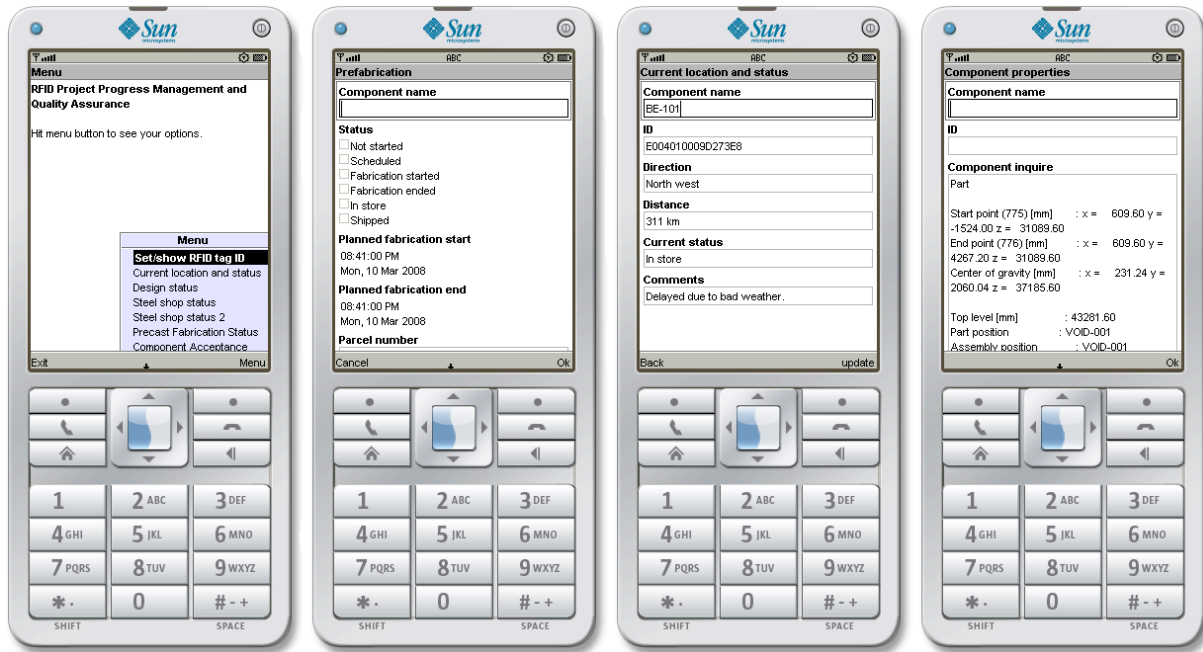
FIG. 15: Screen dumps from a mobile phone based prototype application for project progress management and quality assurance. From left the screen dumps show 1) some of the menu, 2) input window used by the manufacturer of prefabricated components, 3) output from an inquiry of a component's current location and production status, and 4) output from a full component attributes inquiry.
